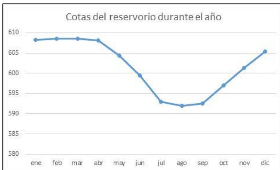
Figure 5-2: Curve of average operation of the reservoir (m at the time).
