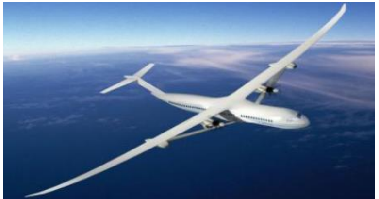
Figure 2 Strut-braced wing (IATA, 2020)
